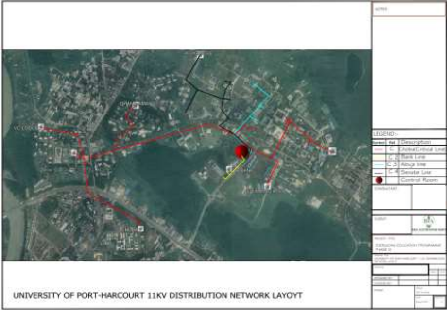
UNIPORT 11KV Distribution Network Layout
