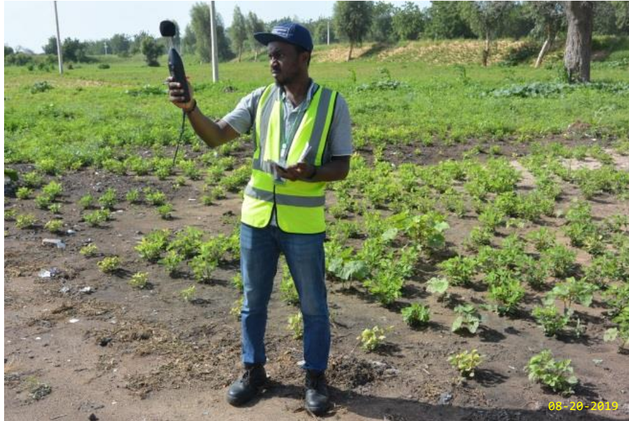
Plate 4.1: Air Quality and noise measurements at the proposed project site
