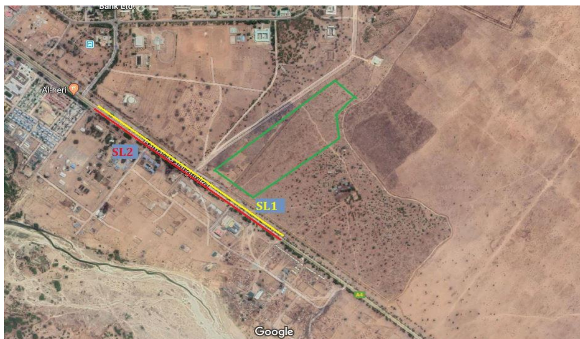
Figure 4.16: Aerial Imagery of the Project site showing the selected screen lines for traffic survey
