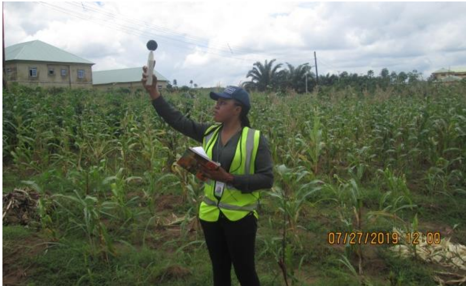
Plate 4.1: Air quality and noise sampling within the proposed project site Source: EnvAccord Field Survey, 2019
