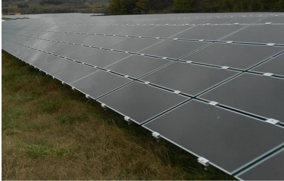
Figure 2.4: Typical appearance of Thin-Film CdTe panels
